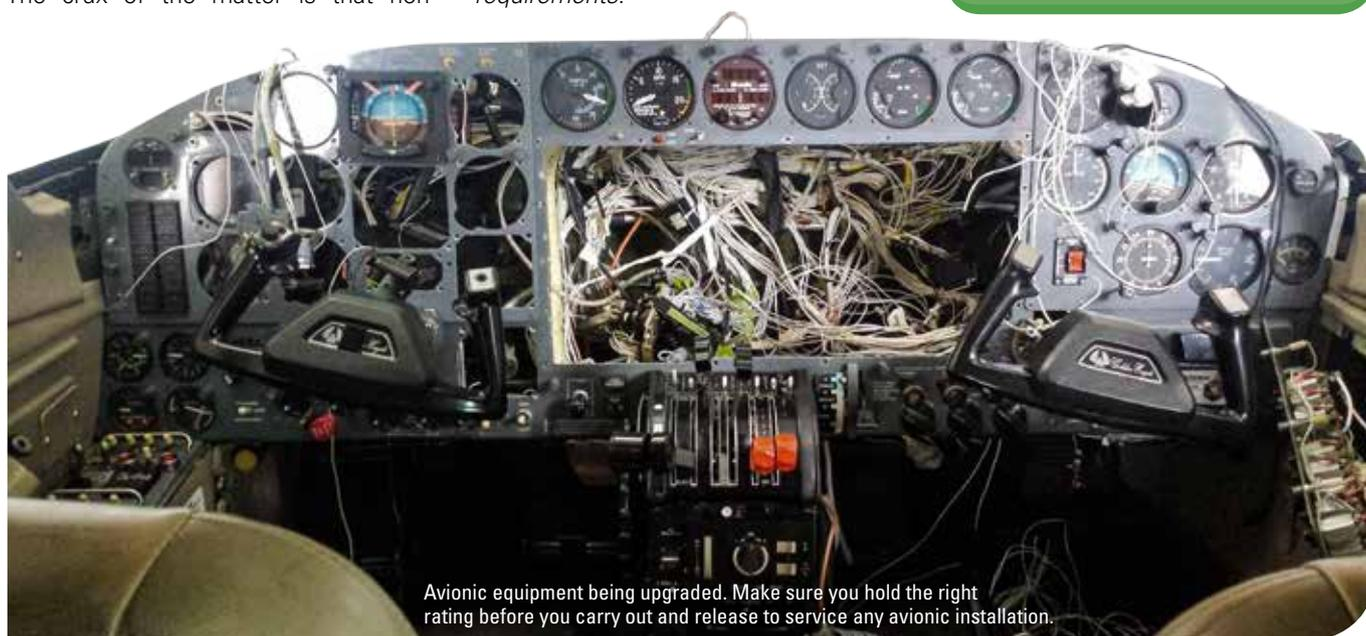
Avionic equipment being upgraded. Make sure you hold the right rating before you carry out and release to service any avionic installation.
