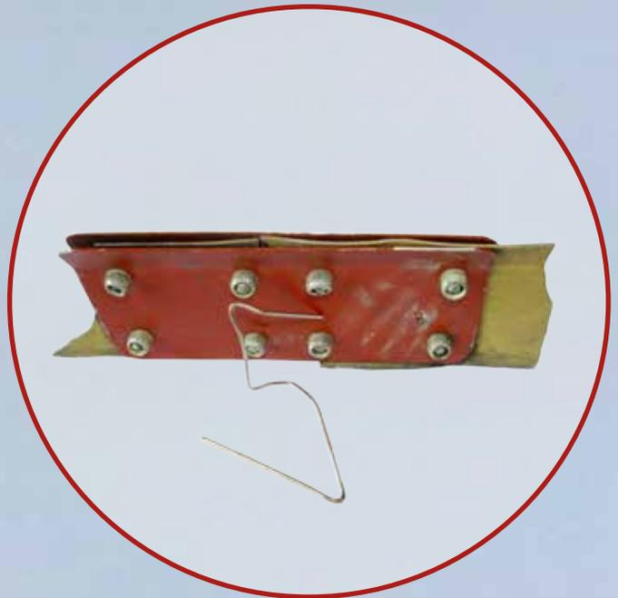
It should have been a minor repair using Acceptable Technical Data. But too much material was used and it resulted in the false spar cracking at each end of the pair.
