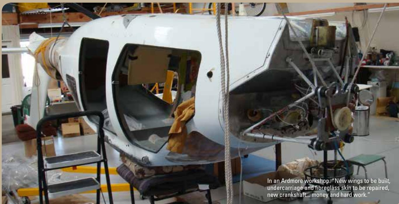
In an Ardmore workshop. "New wings to be built, undercarriage and fibreglass skin to be repaired, new crankshaft... money and hard work."
