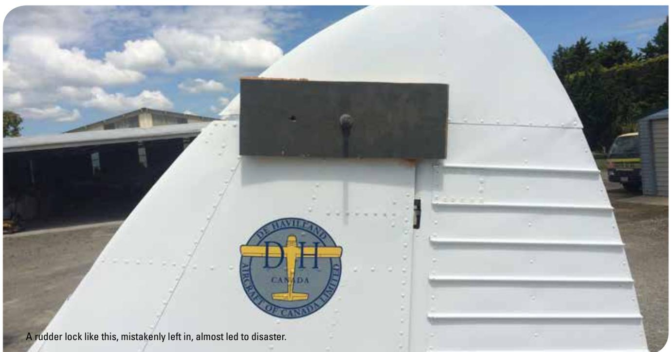
A rudder lock like this, mistakenly left in, almost led to disaster.
