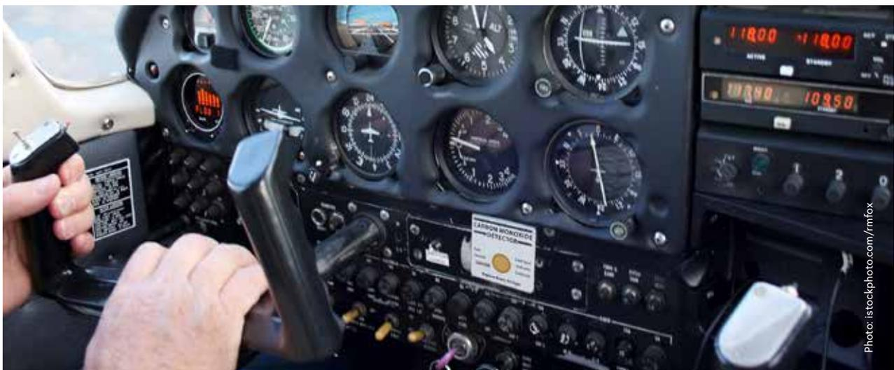
// A view of a cockpit with a carbon monoxide spot detector fitted.
