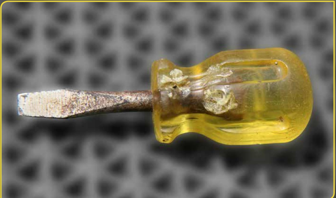
Safety investigators looking into a fatal crash in 2012 concluded that this screwdriver had remained in the rear-most section of the fuselage for some time.
