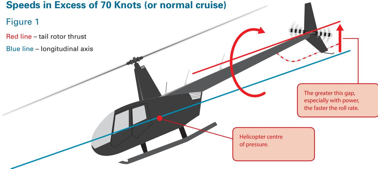
The helicopter encounters a low G condition while in a normal nose down (tail high) cruise. The faster the speed, the higher the tail will be.
