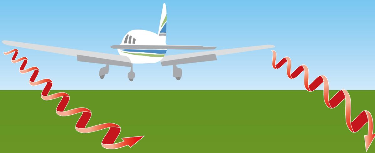
You can't see wake turbulence – just its effects sometimes – and that's what makes it so dangerous. Heavy aircraft aren't the only cause. Sure, you know you don't want to be flying a Cessna in the wake path of an A380, but even light aircraft create wake turbulence.
